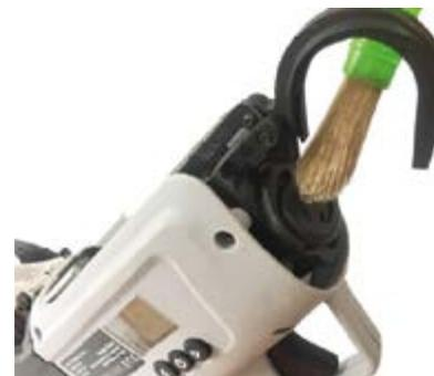
Use a brush to remove foreign objects in the front binding area as shown in the figure
