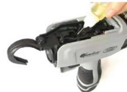
After the cleaning process is complete, lubricate with lubricating oil (ordinary white oil or machine oil) on the cutter and each movable joint as shown in the figure.
