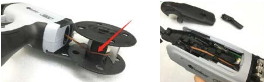
Open the front cover and remove the pressing plate.
