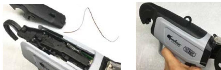
Insert the thread press carriage and place the front cover correctly. The tool can now continue to work with the new thread.
