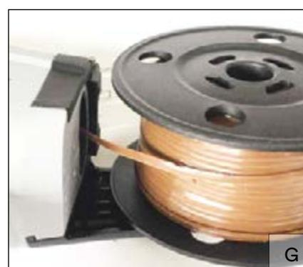
G. Insert the end of the thread into the hole of the machine.
