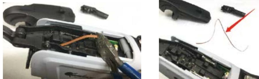
Remove the remaining thread with the tweezers.
