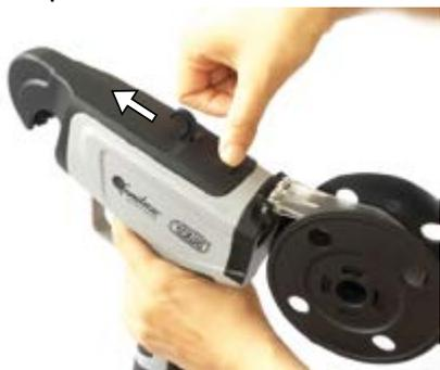
Press the switch to push the front cover if the tool is stuck or unable to power the threads.
